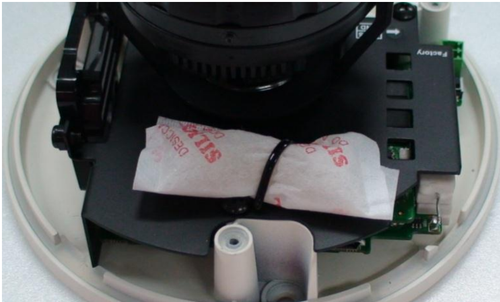
Figure 2-12. Before placing the Dome Cover, remove the silica gel from the PVC bag and install it as shown in the figure for dehumidification. The silica gel should be replaced with new one once it loses the dehumidifying capability.
